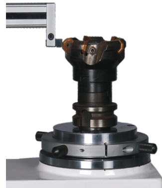
Checking of a Runout
