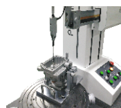
For measuring the roundness on half round bearing
