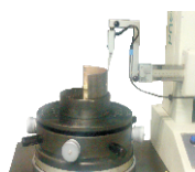
For measuring the roundness on half round bearing
