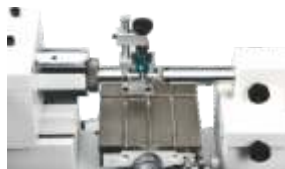
Calibration of Plain Plug Gauge
