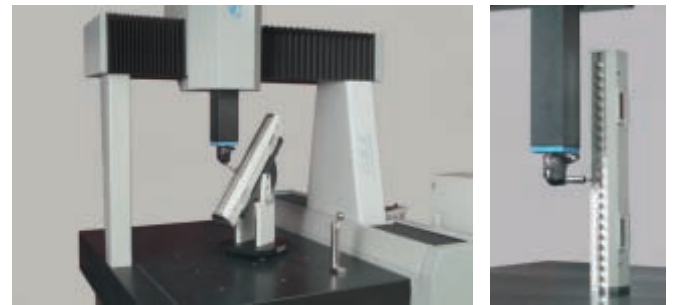
Step gauge for checking the accuracy of co-ordinate measuring machines.
